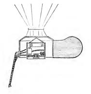
A current passing up by the first wire causes a clockwork apparatus, attached to the camera, to actuate rolls holding the sensitive film in such a manner as to bring a fresh portion of the film behind the lens after an exposure has been made.
